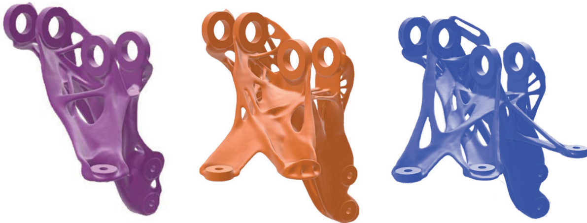
Figure 3: Three different TO results from left to right with more filigree structures. Based on the filigree settings three (rough result – left bracket) up to five (very filigree result – right bracket) attachment points are used. The final design with is developed further is the orange one with four attachment point.
