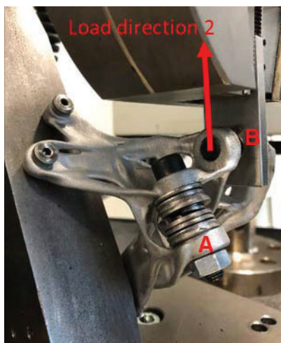
Figure 7 Static validation of the support optimized TO-bracket, Left: the bracket in assembled on the test rig for load 2 attacking in 30° on attachment point B. Load 1 attachment point (A) is bolted together to simulate the additional stiffening connection. Right: Topology optimized bracket test diagram. Test stop without failure at 225 % of the load related to the original (conventional) bracket.
