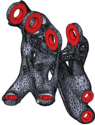
Figure 6 Functional surface of the bracket in red and overview of the brackets during unpacking of the build job
