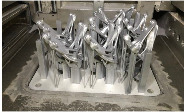
Figure 6 Functional surface of the bracket in red and overview of the brackets during unpacking of the build job
